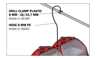
The water supply is made of flexible PE-hoses clicked on to the feeders lid. The hoses can be lead along the vertical feed downpipes, so fewer parts are in the way in the pen and it makes cleaning and installation quick and simple.
