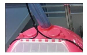
The lid is made with 3 places for feed inlet for optimization of the filling of the hopper, also when using systems with several lines. The arched, dust repellent shape facilitates a maximum filling of the hopper which allows an exact dosage of the feed, even small quantities.
