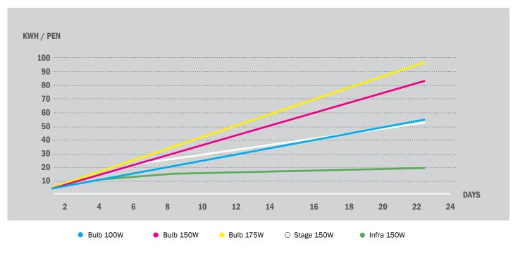
As you can see in the graph, you can save up to 75 kWh/Pen in 23 days by using an INFRA lamp compared to the regular 175W bulb.
