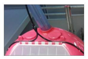
The lid is made with 3 places for feed inlet for optimization of the filling of the hopper, also when using systems with several lines. The arched, dust repellent shape facilitates a maximum filling of the hopper which allows an exact dosage of the feed, even small quantities.
