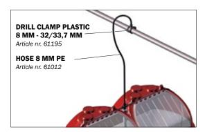
The water supply is made of flexible PE-hoses clicked on to the feeders lid. The hoses can be lead along the vertical feed downpipes, so fewer parts are in the way in the pen and it makes cleaning and installation quick and simple.
