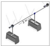
For better stability, we recommend to place the suspension chains every two meters.
