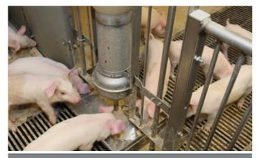
FUNKIMAT is made solely of stainless materials to ensure durability. The FUNKIMAT is designed in consideration of today's demands on housing environment, making the feeder easy to clean as well as waterproof for sprinkling.
